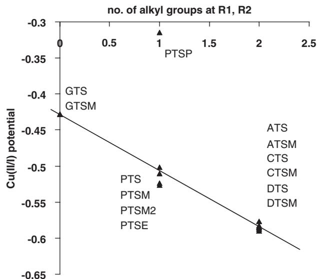
**Figure 2** Effect of backbone alkylation on Cu(II/I) redox potential.
